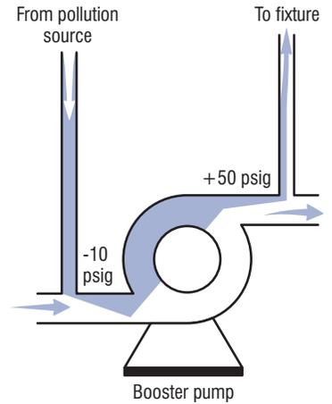
flow from the source of pollution would occur when pressure on the suction side of the pump is less than pressure of the pollution source; but this is *backflow*, which will be discussed below.
