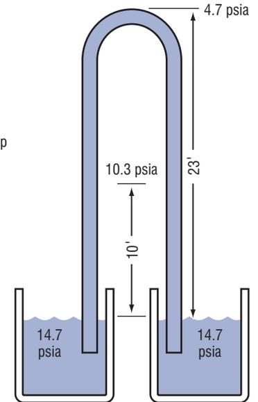
above the level of the other. (See Fig. 6.) Since both containers are open to the atmosphere, the pressure on the liquid surfaces in each container will remain at 14.7 psia.
