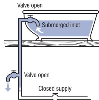
The siphon actions cited have been produced by reduced pressures resulting from a difference in the water levels at two separated points within a continuous fluid system.
